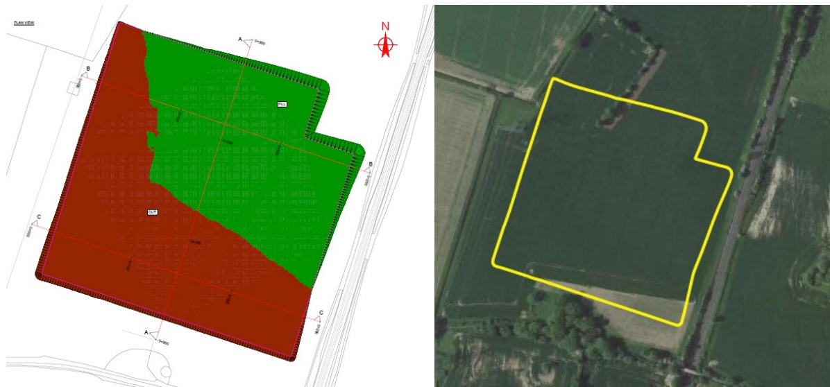
Figure 9-129-12: Extract of the Cut and Fill Drawing (left) and Option 2 with Embankments z-shape used in model
